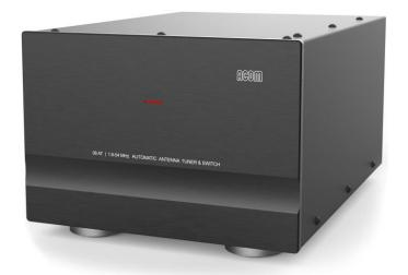
ACOM 06AT automatically selects one of four available antenna outputs (as assigned in bands by the operator) and matches the impedance of the chosen antenna output by transforming it to 50 Ohm with SWR below 1.5:1 at the tuner input (typically below 1.3), providing an optimum load impedance for the amplifier.
