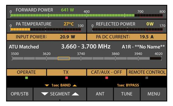
Figure 3-1 | ACOM 700S amplifier screen with tuner installed
