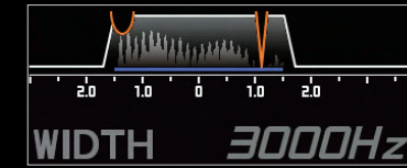
IF DSP Operating Status Display
