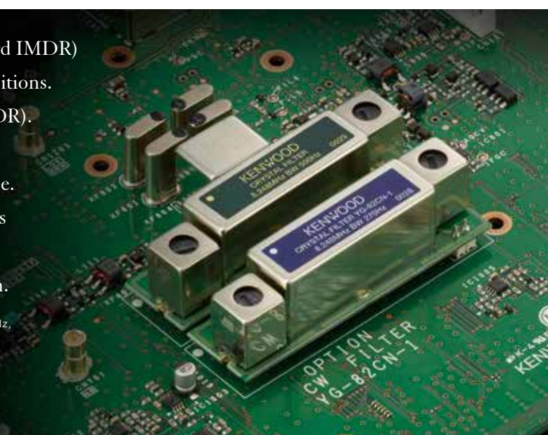
Photograph shows optional 270Hz roofing filter installed.
