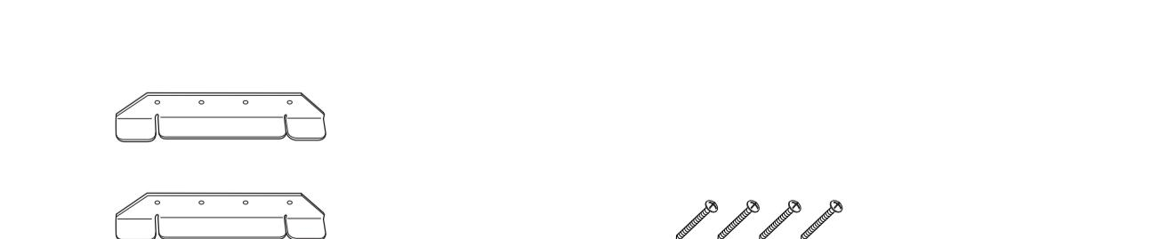
Attach these brackets when locating the keyboard away from a wall.
