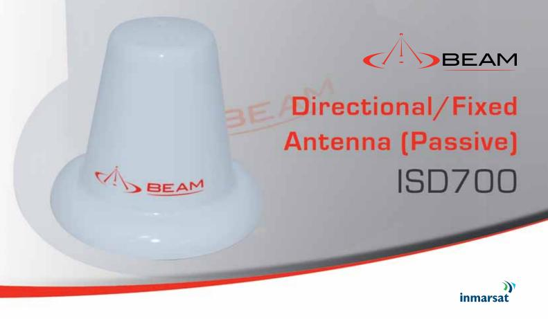
BEAM Directional/Fixed Antenna (Passive) ISD700 is a dual mode Inmarsat & GPS antenna, designed predominantly for land. The ISD700 dual mode directional/fixed antenna is supplied with U-bolts that enables it to be securely mounted on to a pole. The directional/fixed antenna is fitted with an SMA female connector for GPS and a SMA for Inmarsat.
